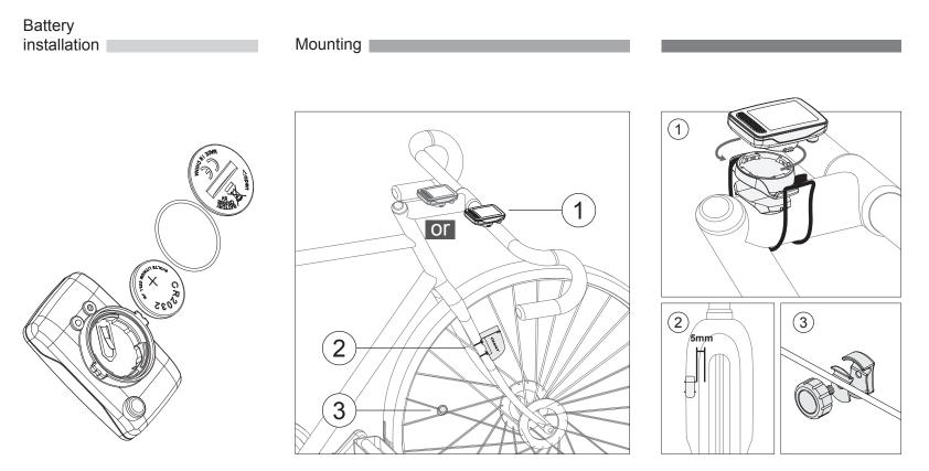
Install the battery in the back of the main unit. Use a coin to open and close the cover.
