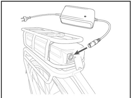
**With the EnergyPak removed from the bike.**
