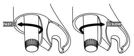
The adjustment range is from slowest position which turns rebound damper knob completely clockwise to fastest position which turns rebound damper knob completely counterclockwise.
