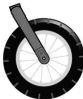
Figure 2 Insert axle into the fork
