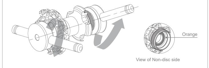
After every bearing replacement, please glue the bearing into the hub shell by using Loctite 290 and dry for 24+ hours. Pay special attention not to let excess Loctite dry on the waterproof cover. Clean off excess glue immediately.
