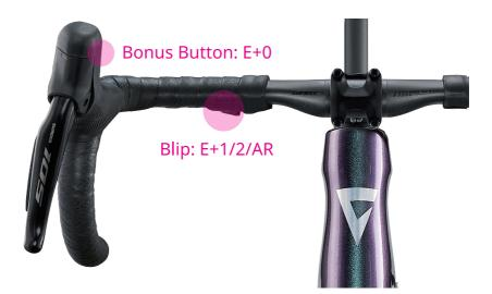
Sram AXS Bonus Button/Blip is the integrated remote button for an intuitive drop-bar control. In our E-system, we can use them for switching the assist level during the ride.
