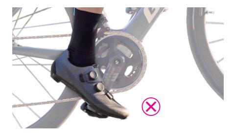
For the best riding experience, torque sensor has to be calibrated on every ride. Please **Do not** put your foot on the pedal while switching the system on. When pressure is applied during switch on the bike needs more time to calibrate, possible resulting in different ride feeling temporarily.
