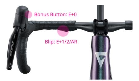
AXS Blips and Di2 buttons can be configured to adjust this bike's assist level while riding. The default configuration is as follows:
