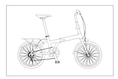
2. Open the seat post clamp and lower the seatpost to its lowest possible position.
