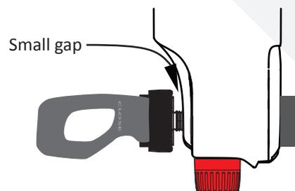
4. If the lever is too tight to close, do not force it, remove the thru-axle and adjust the indexed nut on the non-drive side of the fork by one increment in a counter-clockwise direction. Repeat as necessary until the lever closes smoothly and firmly.
