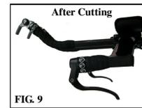
The Tri-bar should be clamped securely in a vice before cutting. To accommodate this without cracking the bar, the bar should be held in a tubing fixture. You can make this fixture quite easily by boring a 23.8mm diameter hole in a 4" section of 2" x 4" and then cutting the block in half. The two blocks can then be placed into the vice to hold the bar firmly in place. A similar functional clamp can also be used for this purpose. Be careful not to over tighten the vice.
