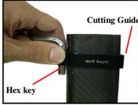
Prop the Cutting Guide open with a hex key. Then, install the Cutting Guide onto the integrated seat post.
