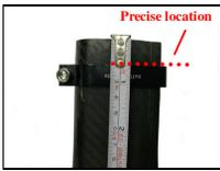
Place the Cutting Guide to the precise location of the desired cut. Be sure to double-check your measurement. Rechecking measurements is easier than buying another ISP frame.
