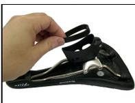
Step 4: Install the saddle onto the seat post.
