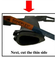
**⚠ CAUTION:** To avoid fraying the composite fibers. Using a fine tooth (32 teeth) saw blade is recommended.
