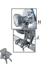
3. The Linkage pillar "J" is controlled by the Wheel Adjustment Knob "H". Try to move linkage pillar from frame attachment stay tracking location (a) to (b) until it's locked.
