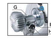
8. Before proceeding make sure that the rear tire of the bike is properly inflated. Check the sidewall of the tire for the manufacturer's recommended pressure range, and inflate accordingly. Using the Adjustment Knob "H" set the Fluid Resistance Unit "I" so that the roller contacts the bike's rear tire. Then turn the Adjustment Knob "H" clockwise two full turns to insure that you have sufficient pressure of the Drive Roller "G" on the rear tire.
