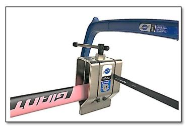
**NOTE!** To avoid fraying the composite fibers. Use a fine tooth (32 tooth) saw blade.
