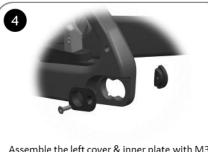
Assemble the left cover & inner plate with M3 bolt at the rear of the dropout.
