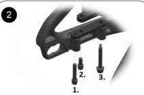
Mount the brake caliper and bracket with 3 bolts in indicated sequence (1. medium, 2. short, 3. long).
