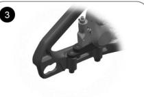
Tighten the 3 M5 bolts. Tightening torque: 6 ~ 8 N-m.
