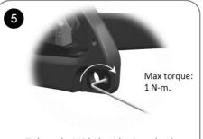
Tighten the M3 bolt with a 2mm hex key.
