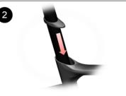
Insert the seatpost into the frame.
