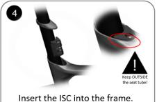
Insert the ISC into the frame. Keep the ridge outside the seat tube.
