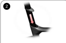
Insert the seatpost into the frame.
