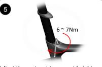
Adjust the seatpost to correct height and tighten the ISC bolt with a 4mm hex key.
