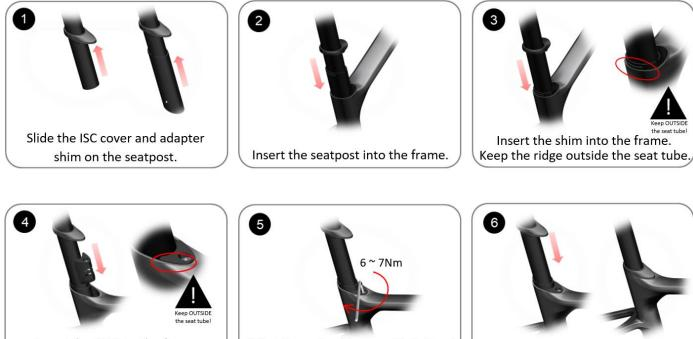
Insert the ISC into the frame. Keep the ridge outside the seat tube. Adjust the seatpost to correct height and tighten the ISC bolt with a 4mm hex key.
